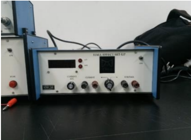
FIG. 4: The Hall effect experiment setup consisting of a constant current provider and a digital millivoltmeter.
