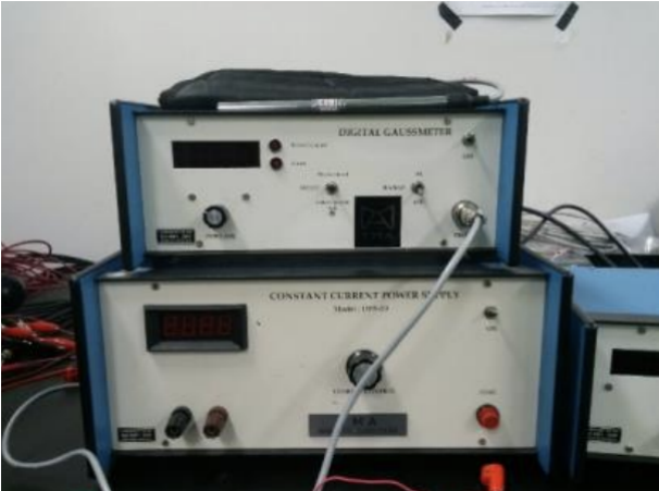
FIG. 1: A digital Gauss meter and a constant power supply (for the electromagnet [4]).
